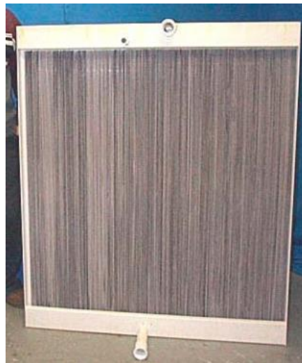
Figure 11 A 6,000 cfm low-flow liquid-desiccant conditioner 41
