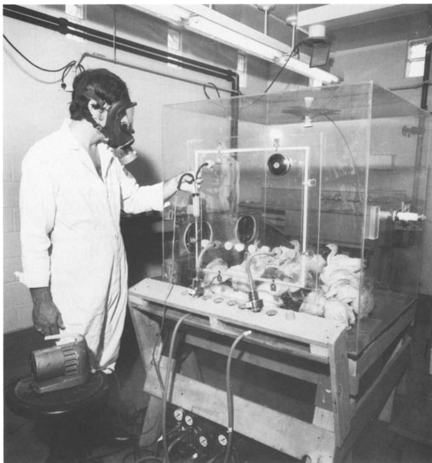
Fig. 2. Exposure chamber and apparatus for exposure of turkey poults to aerosols of fungal spores (12).
