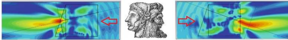
Fig. 2 The particle with broken symmetry for PH formation: the morphology of the field localization area depends on the orientation of the particle that resembles the two faces of “Janus bifrons”. Adapted from Ref. [33].
