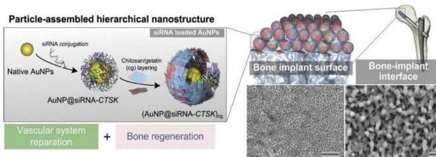
FIGURE 10 | siRNA-decorated nanoparticles were assembled to engineer a hierarchical nanostructured coating on clinically used titanium implants for the synergistic regeneration of skeletal and vascular tissues. Reproduced from Xing et al. (2020) with permission from Elsevier (Copyright 2020).
