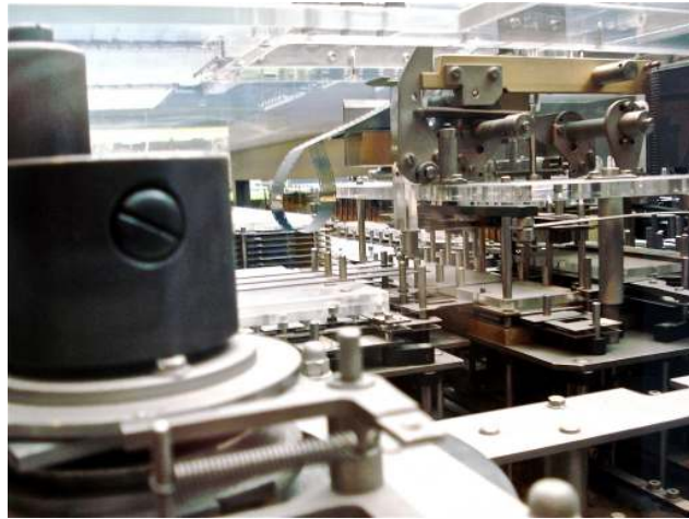
Figure 75: Replica of the first mechanical computer designed by Konrad Zuse, the Z1, finished in 1938. It was a binary electrically driven mechanical calculator which used Boolean logic and binary floating point numbers. Picture taken by H. Zenil, Deutsches Technikmuseum (“German Museum of Technology”), Berlin.
