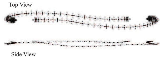
Fig. 1. Simulation results of two quadrotors reciprocally avoiding collisions while exchanging positions with each other. The quadrotors choose to avoid collisions by passing beside each other.
