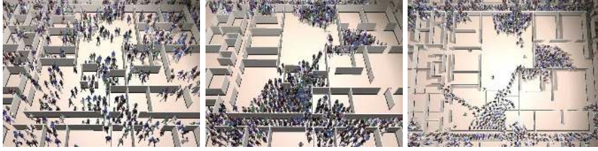
Fig. 9 Snapshots from simulation of 1,000 virtual agents evacuating an office as part of a crowd simulation.
