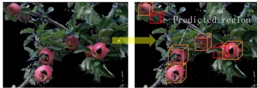
FIGURE 9 | Apple identification implemented via RGB-D camera and SVM classifier (Tao and Zhou, 2017).
