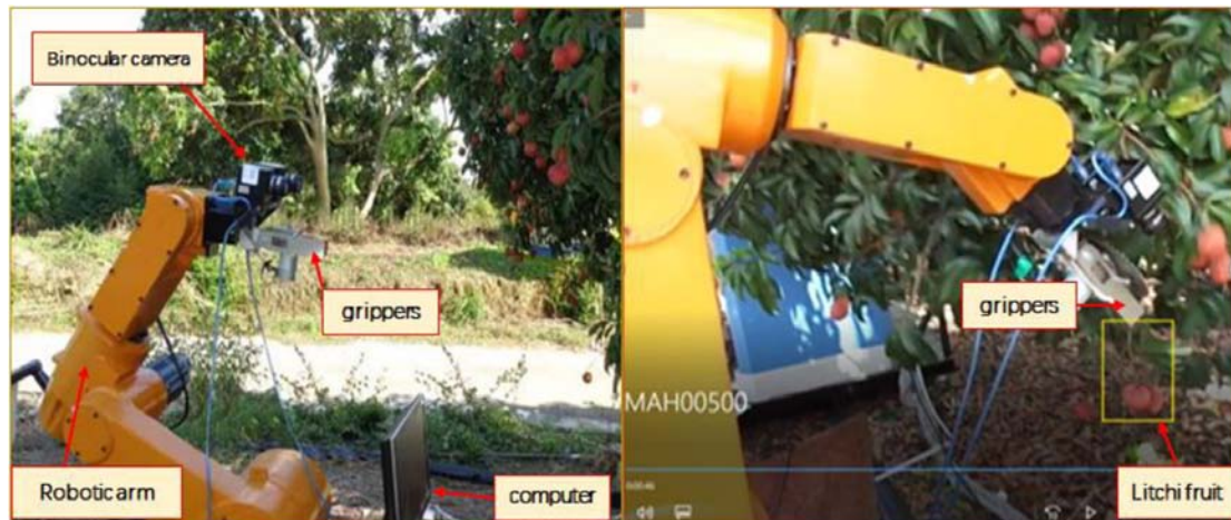
FIGURE 5 | Litchi picking robot based on binocular stereo vision.
