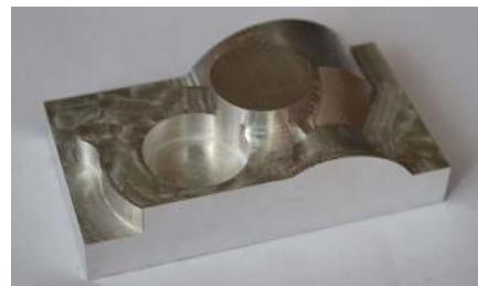
Fig. 5. The test piece used in case study 1 – machined part with planar surfaces parallel to coordinate axes.
