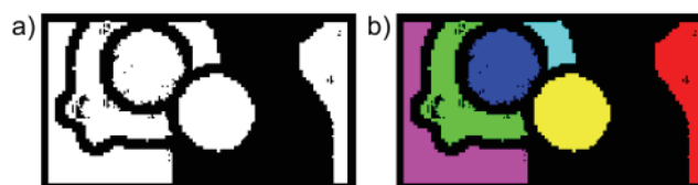
Fig. 6. a) Binary image after details thresholding; b) Detected connected regions in binary image.
