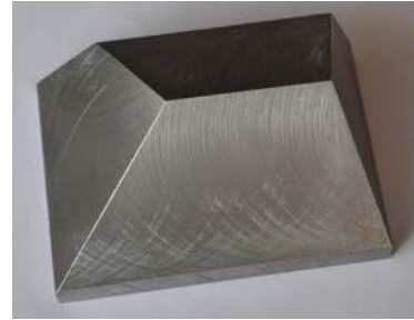
Fig. 8. The test piece used in case study 2 – machined part with planar surfaces with arbitrary orientation.
