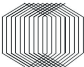
Fig. 10. Scheme of rotor windings of the healthy DC motor
