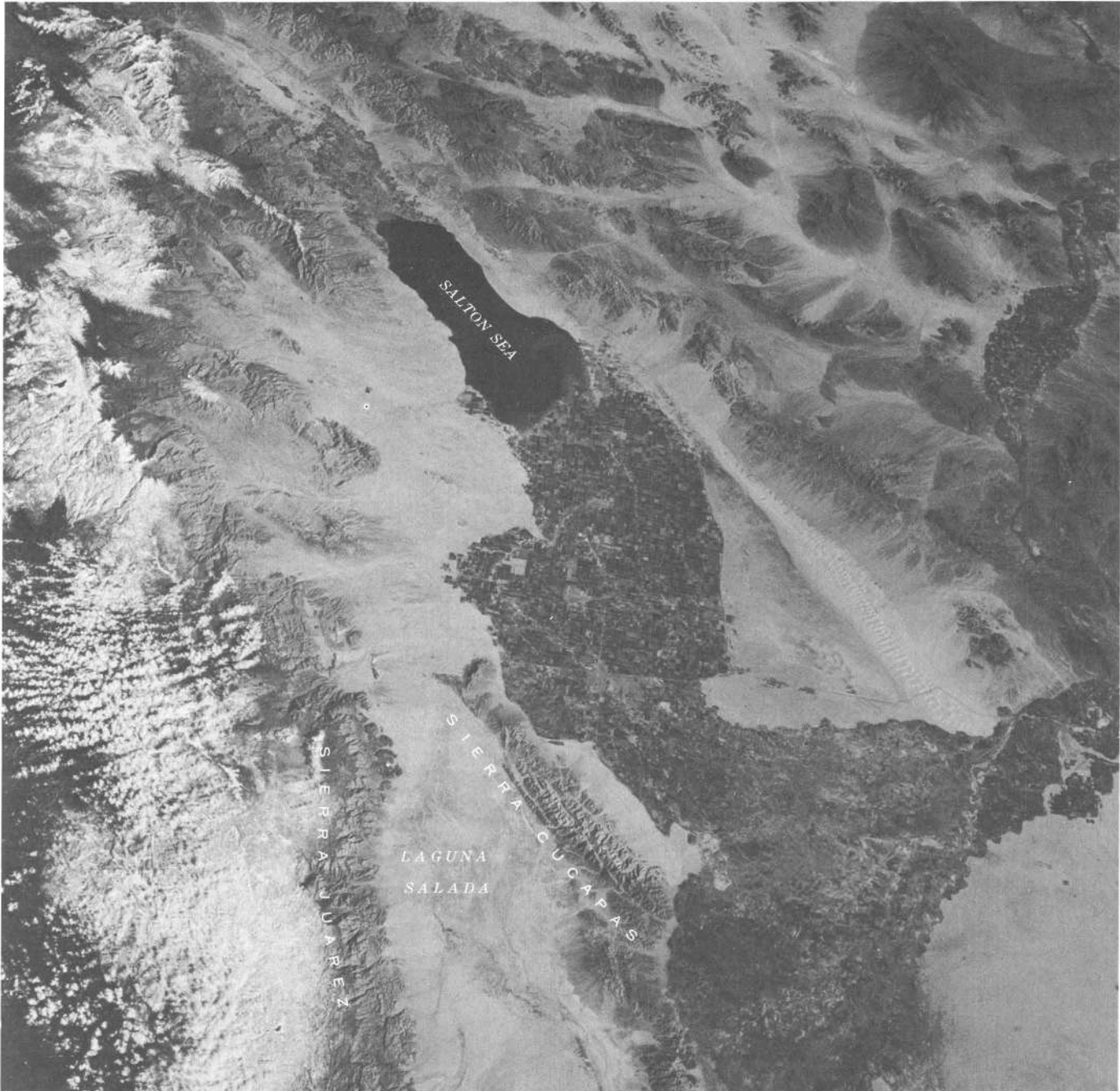
FIGURE 6. — Photograph looking steeply downward at the Salton depression, southern California and northern Baja California. The aligned canyons of the Sierra Cucapas (lower center) mark strike-slip faults. The high normal-fault scarp of the Sierra Juarez is obvious at lower left. The San Andreas fault trends northwestward (toward upper left, across upper third of picture) but is not apparent on the photograph. The ranges northeast (above and right) of the San Andreas may be outlined primarily by strike-slip faults, but these cannot be identified in the picture. Apollo 9 photograph AS9-23-3558, 11 March 1969.
