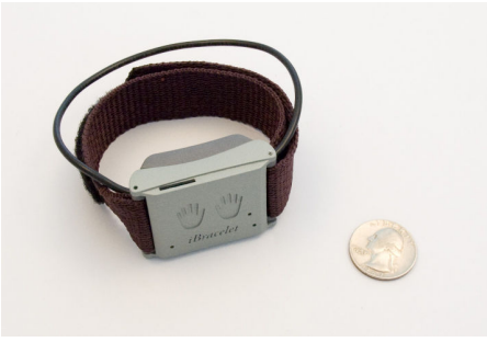
Figure 12. The iBracelet wrist-worn RFID reader. To facilitate comparison with WISPs (which do not require any wearables), we tagged our objects with both stock RFID tags and WISPs. We required all subjects to wear an iBracelet on their dominant hand. Subject activity resulted in synchronized streams of object-use data from iBracelets and WISPs.
