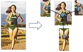
Figure 6. The four part star structured model. We divide the pose into four parts: legs, left-arm, right-arm, and upper-body.
