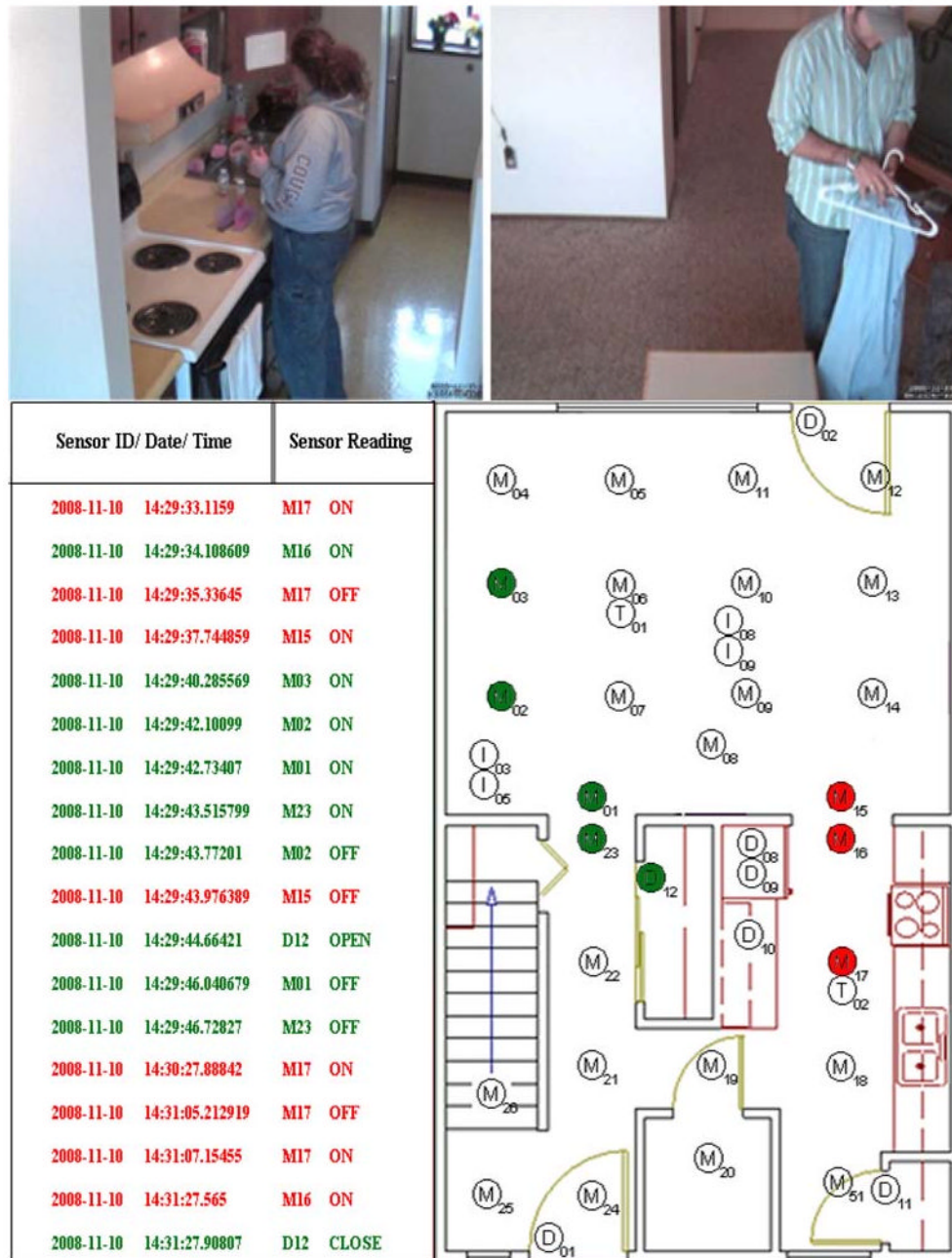
Fig. 2. Multi-resident participants performing activities in smart apartment. Person A ( upper left ) is performing “Fill medication dispenser” activity while Person B ( upper right ) is performing “Hang up clothes” activity. The sensor events corresponding to these activities is shown in the lower left and is visualized in the lower right
