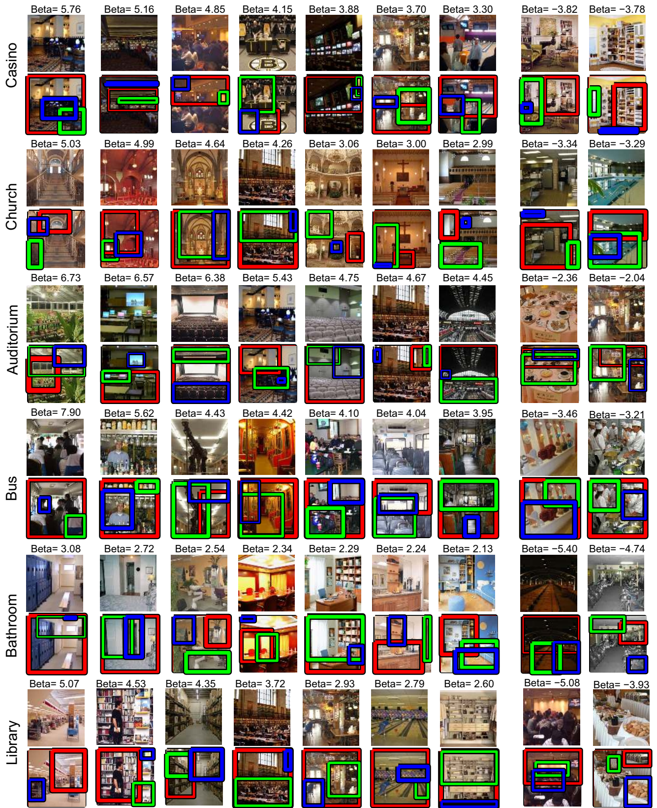
Figure 9. Prototypes for a subset of scene categories and sorted by their weight. The 7 first columns correspond to the highest rank prototypes and the last two columns show prototypes with the most negative weights. The thickness of each bounding box is proportional to the value of the weight for each ROI: \lambda_{kj} .
