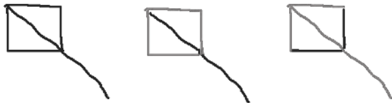
Figure 12: The left shows the originally drawn strokes. The middle interpretation is made up of a line and a square. The right interpretation is made up of an arrow and two lines.
