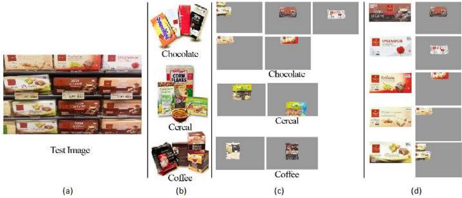
Fig. 1. System overview: (a) Given a test image, (b) we first filter the categories that the test image may belong to, (c) then we match the test image against all images in the filtered categories. (d) An energy function is then optimized given the top-ranked matches to obtain the final list, along with inferred locations, of recognized products.
