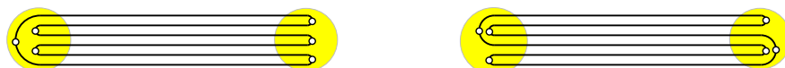
Figure 3: Two perturbations of a weakly simple polygon on 6 vertices (all of them spurs) that alternate between two distinct points in the plane.
