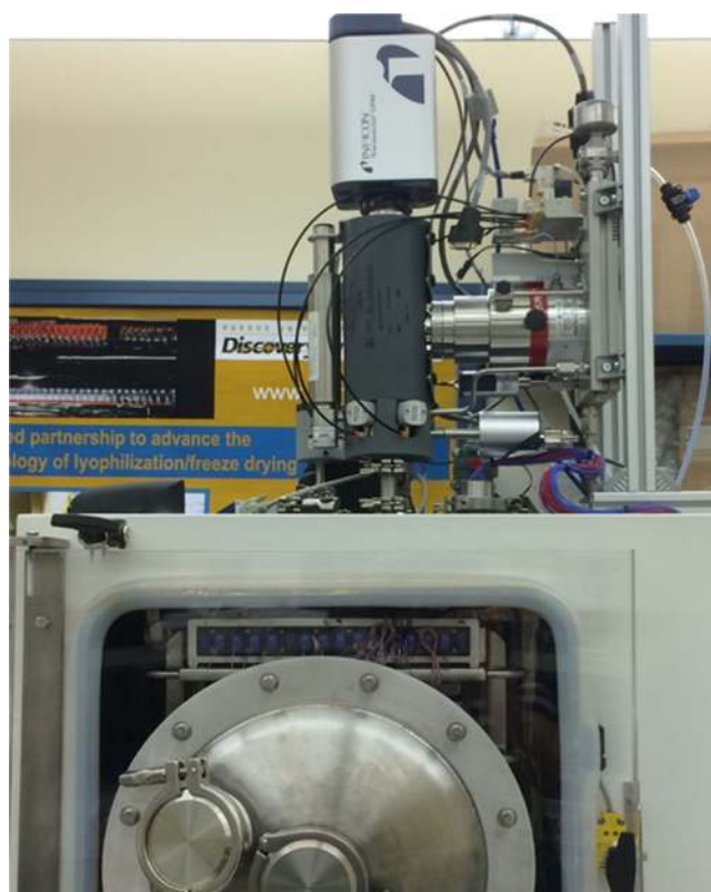
Fig. 12. Quadrupole mass spectrometer installed on a laboratory-scale freeze dryer for in situ monitoring of gas composition in the product chamber
