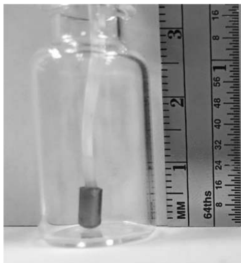
Fig. 4. Vial containing a 100 ohm platinum RTD sensor
