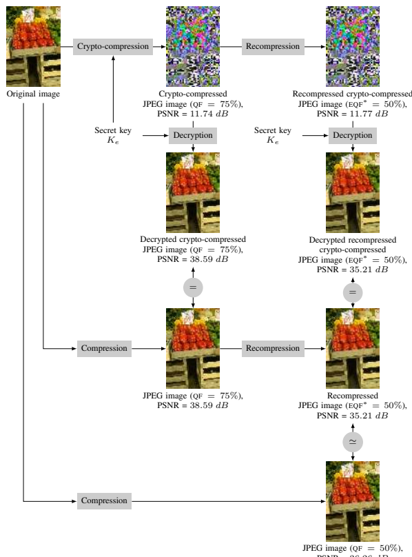
Fig. 9: Full application example of our proposed method: crypto-compression of the Peppers image ( QF = 75\% , encryption of both AC and DC coefficients of the luminance and two chrominance components) and recompression of the crypto-compressed image ( EQF^* = 50\% ).
