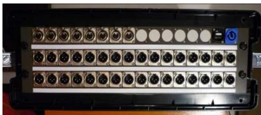
Figure 10. Final system MIAUDIO in the box with all the required input/output connectors.
