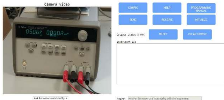
Fig. 3. Main web interface GPIB SCPI experience
