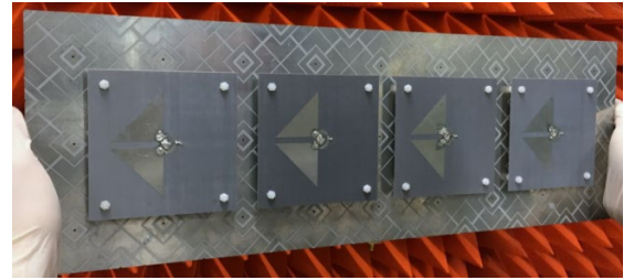
Fig. 9. Fabricated prototype of the 1 \times 4 CP reconfigurable antenna array
