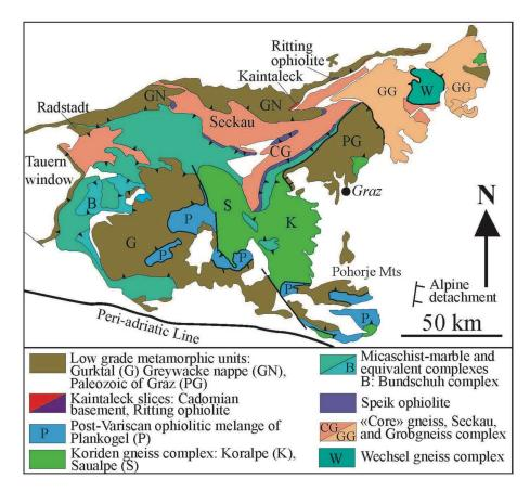
**Figure 9.** Tectonic map of the Austroalpine Domain east of the Tauern window. The Ritting, and Speik ophiolites subdivide the Variscan units into three main groups, namely: (i) the low-grade metamorphic units (Gurktal nappe, Greywacke nappe, and Paleozoic of Graz), (ii) the Koriden gneiss, and Micaschist–marble complexes, and (iii) the "Core" gneiss, Grobgneiss, and Wechsel gneiss complexes (simplified from [118]). For the interpretation of nappe architecture, see Figures 10 and 11.
