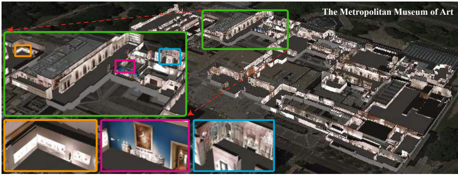
Fig. 1. A texture mapped 3D model of The Metropolitan Museum of Art reconstructed by our system, which directly recovers a constructive solid geometry model from 3D laser points.
