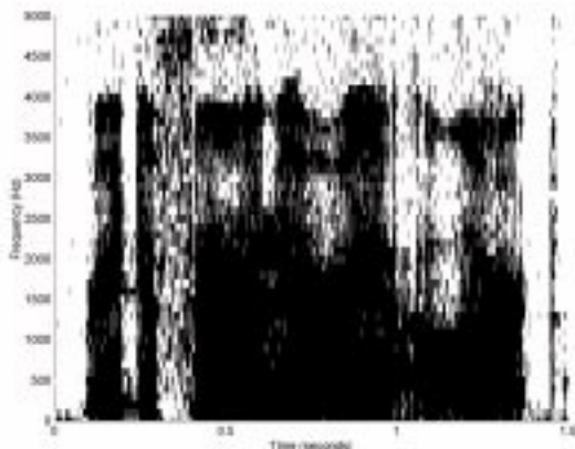
Figure 3.4 Quantized spectrogram of an utterance of speech that has been corrupted to 20 dB by additive white noise. All regions of the spectrogram where the local SNR is greater than 0dB ( i.e. where the speech energy was greater than the noise energy) are colored black. All regions with local SNR less than 0 dB are colored white. Only frequencies up to 5 KHz have been shown in the figure.
