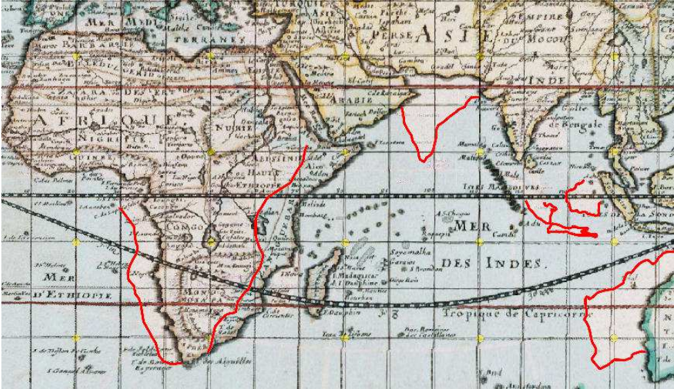
Figure 6.4. A comparison of the analyzed map in the Nicolosi globular projection re-projected to the Mercator projection and the outlines of the continents in Open Street Maps; the continents are stretched in the east-west direction.
