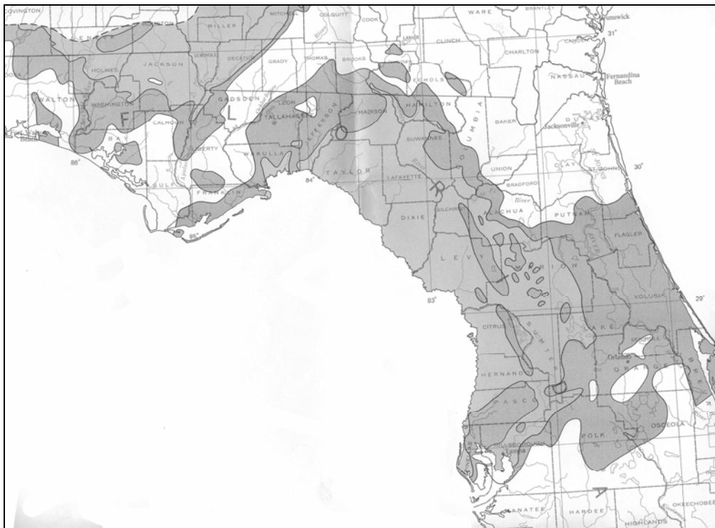
Figure 3.1: The Floridan Aquifer System in the Study Area. Light gray: unconfined; dark gray: semi-confined, and white: confined. Adapted from Bush and Johnson (1988:plate 2).
