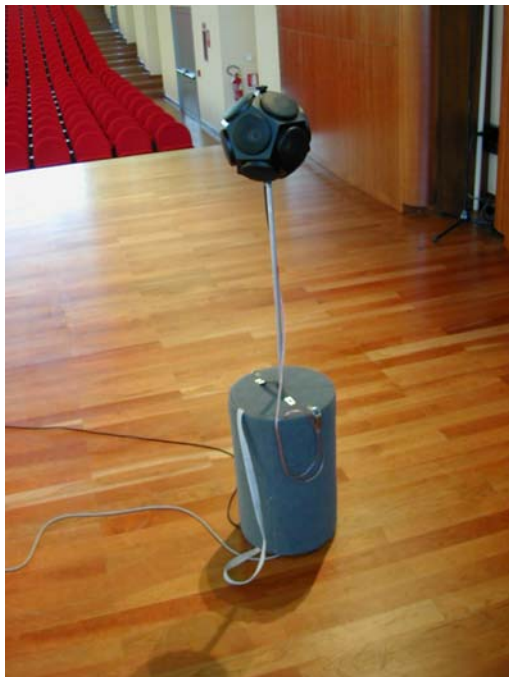
Figure 4: Dodechaedron loudspeaker and subwoofer.
