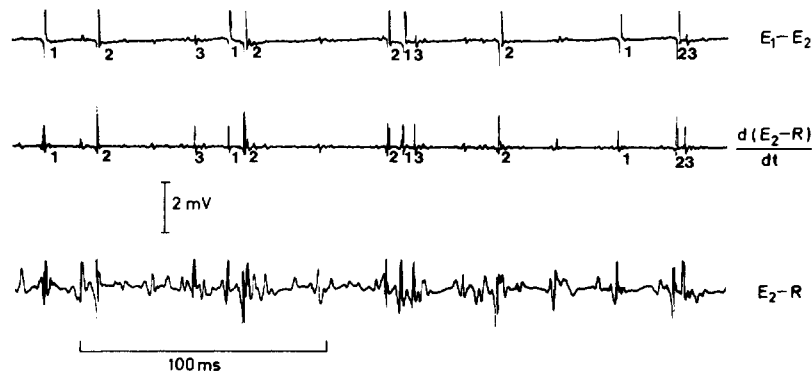
Fig. 11. Above: Selective recording of action potentials from two motor units 1 and 2 via a side hole electrode in the anterior tibial muscle of a normal subject at 20% of maximal effort. Middle: Action potentials from three motor units (1, 2, and 3) selected by differentiation of the lower trace: d(E_2 - R)/dt . Note the similar shape of the potentials from motor units 1 and 3. Below: Summated activity from many motor units recorded between one of the recording surfaces of the side hole electrode and a reference electrode ( E_2 - R ).
