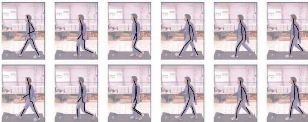
Fig. 8. Comparison between single exemplar and dynamic programming. The top row shows results obtained matching to a single exemplar and the bottom row uses dynamic programming to combine limbs from multiple exemplars. The third column shows an example of reuse of edge pixels to match left and right legs at same location.
