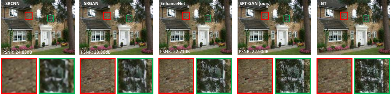
Figure 2. Comparing different SR approaches with downsampling factor \times 4 : SRCNN [7], SRGAN [27], EnhanceNet [38], our proposed SFT-GAN and the original HR image. SRGAN, EnhanceNet, and SFT-GAN clearly outperform SRCNN in terms of perceptual quality, although they yield lower peak signal-to-noise ratio (PSNR) values. SRGAN and EnhanceNet result in more monotonous textures across different patches while SFT-GAN is capable of generating richer and visually pleasing textures. ( Zoom in for best view ).
