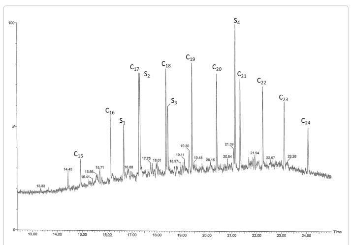
Figure 1: GC-MS chromatogram of oil extracted from COTBS with some selected peaks identified. S1 2,6,10-trimethyldodecane, S2 2,6,10,14-tetramethylpentadecane, S3 2,6,10,14-tetramethylhexadecane, S4 cyclic octa-atomic sulphur.
