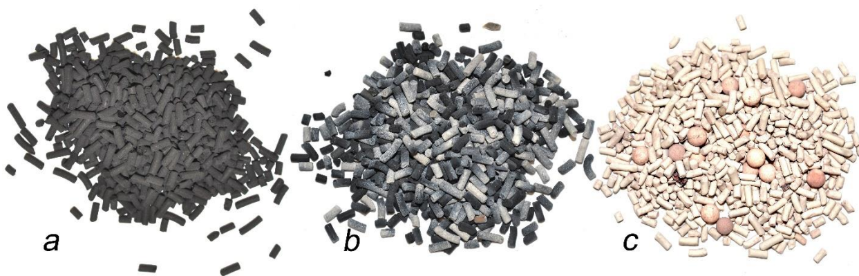
640 641 Figure 11. Spent catalyst Pt/ Al 2 O 3 : a) before sintering, b) after 10 minutes of calcining at 800 °C, c) after 642 30 minutes of calcining at 800 °C with manual stirring
