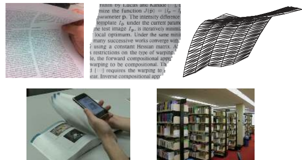
Figure 1. First row: From a single image of smoothly curved document as input, our methods compute the 3D shape of the document and a rectified image of text with no warping or shading effects. Second row: Two potential applications of our system: mobile text scanning and book digitization. (Images from Google).
