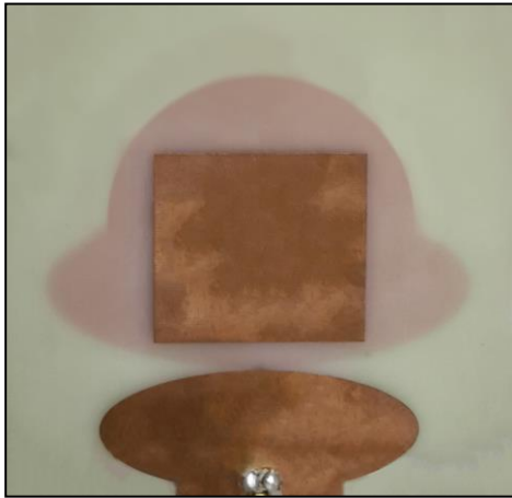
Fig. 1. Fabricated hat patch Microstrip antenna [4]
