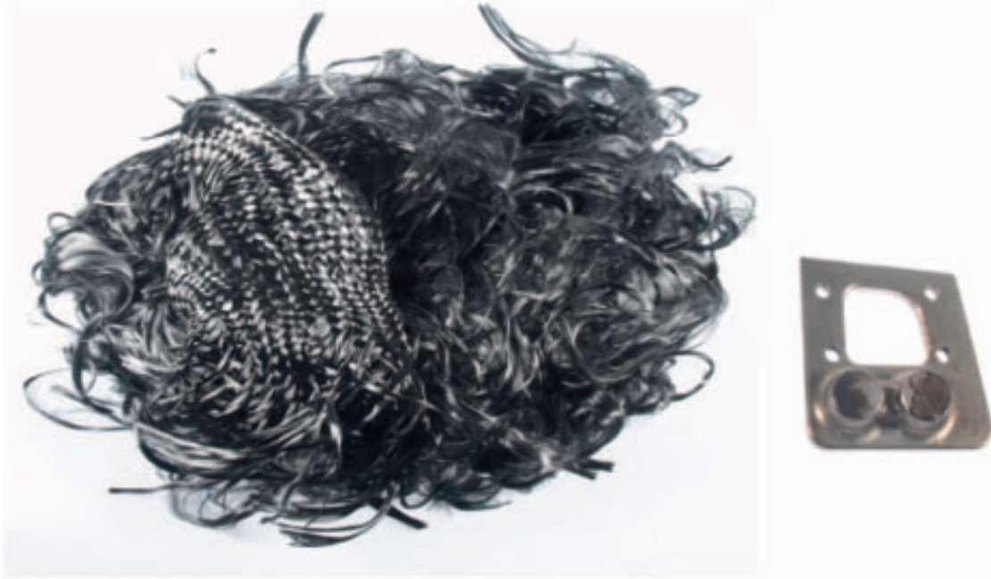
Figure 4. Carbon fiber reinforcements after acid digestion (a) and separation of aluminum insert (b); the fibers appear mostly as single tows, but in a few places, the twill architecture is still visible.
