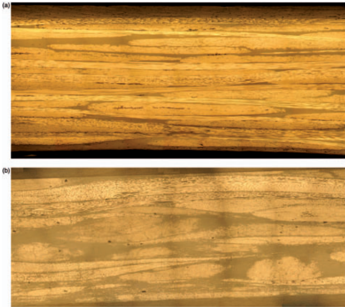
Figure 10. Optical microscopy images of a vacuum-assisted resin transfer molding (VaRTM) panel manufactured using the pristine twill reinforcement (A) and the one using the recycled long random fiber reinforcement (B).
