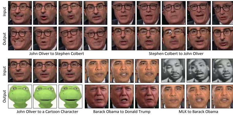
Fig. 5. Face to Face: The top row shows multiple examples of face-to-face between John Oliver and Stephen Colbert using our approach. The bottom row shows example of translation from John Oliver to a cartoon character, Barack Obama to Donald Trump, and Martin Luther King Jr. (MLK) to Barack Obama. Without any input alignment or manual supervision, our approach could capture stylistic expressions for these public figures. As an example, John Oliver’s dimple while smiling, the shape of mouth characteristic of Donald Trump, and the facial mouth lines and smile of Stephen Colbert. More results and videos are available on our project webpage.
