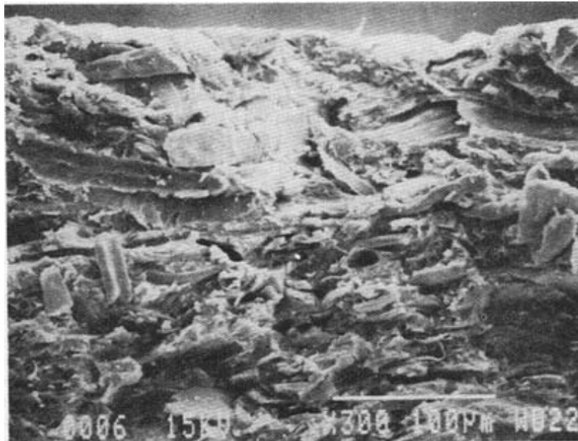
Figure 2. SEM of the fracture surface (notched Izod test) of the uncoupled composite showing some fiber pull-out and topographical uneven surface.
