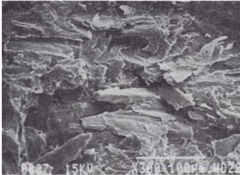
Figure 4. SEM of the fracture surface (notched Izod test) of the E-43 coupled composite showing little fiber pull-out.
