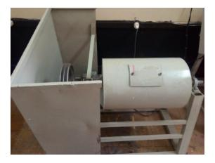
Fig. 3. Bug-milling machine
