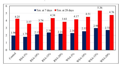
Fig. 11. Tensile strength at 7 & 28 days
