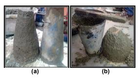
Fig. 6. Slump test; concrete a) without Superplasticizer, b) with Superplasticizer
