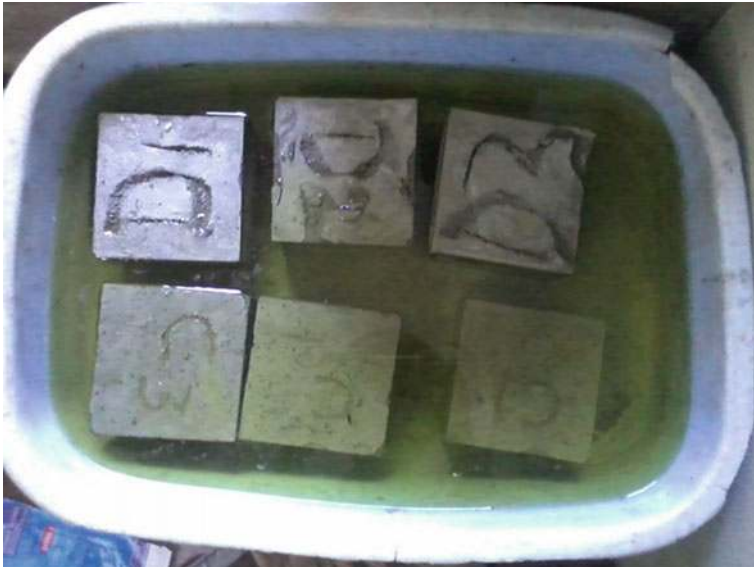
Fig. 3 Curing of S/S mortar blocks
