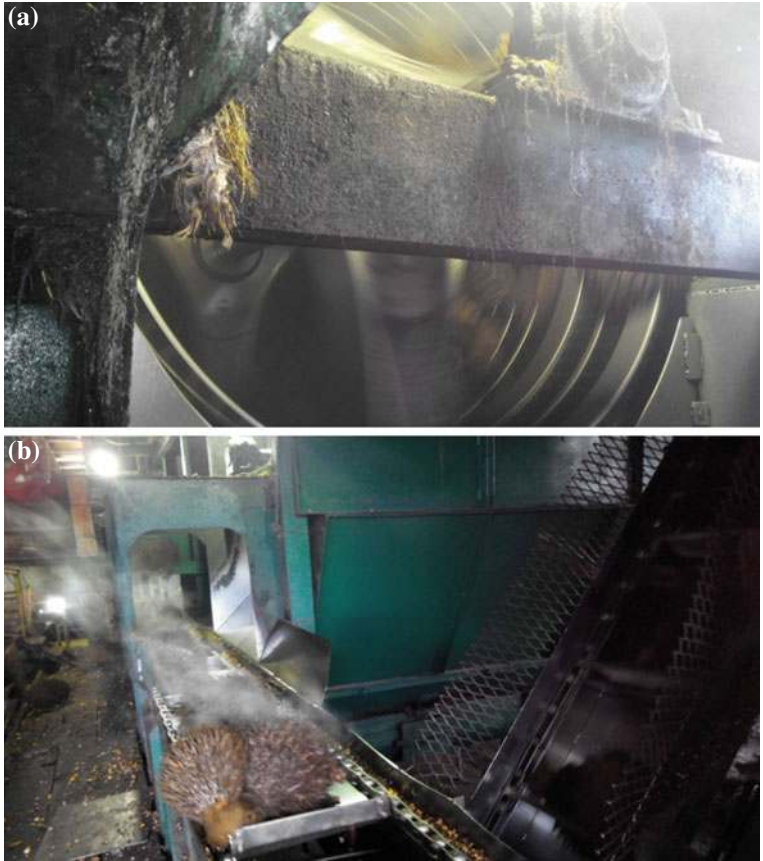
Fig. 4 Revolving slated steel drum for fruit recovery (a) and palm oil drum strippers (b)
