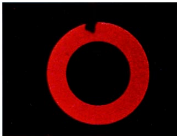
FIG. 1. Photograph of red emission from a ring structure ITO/GaN:Eu LED of area 7.65×10 −4 cm 2 and ring width of 75 μm, operating with 50 V and 0.6 mA. The dark notch in the upper part of the ring is caused by the probe tip obscuring the emission.
