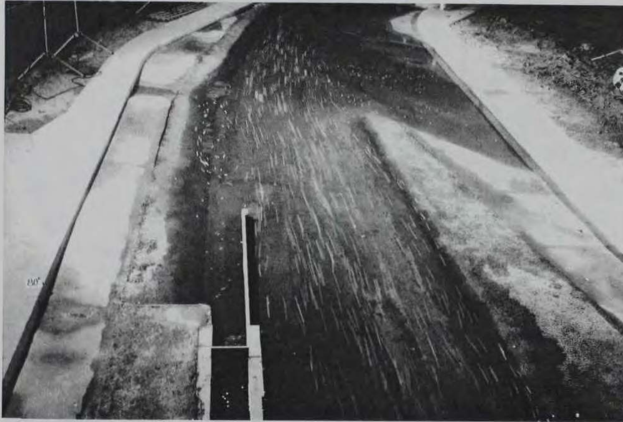
Photo 38. Plan D-2, looking downstream, discharge 80,000 cfs. Confetti showing surface current patterns
