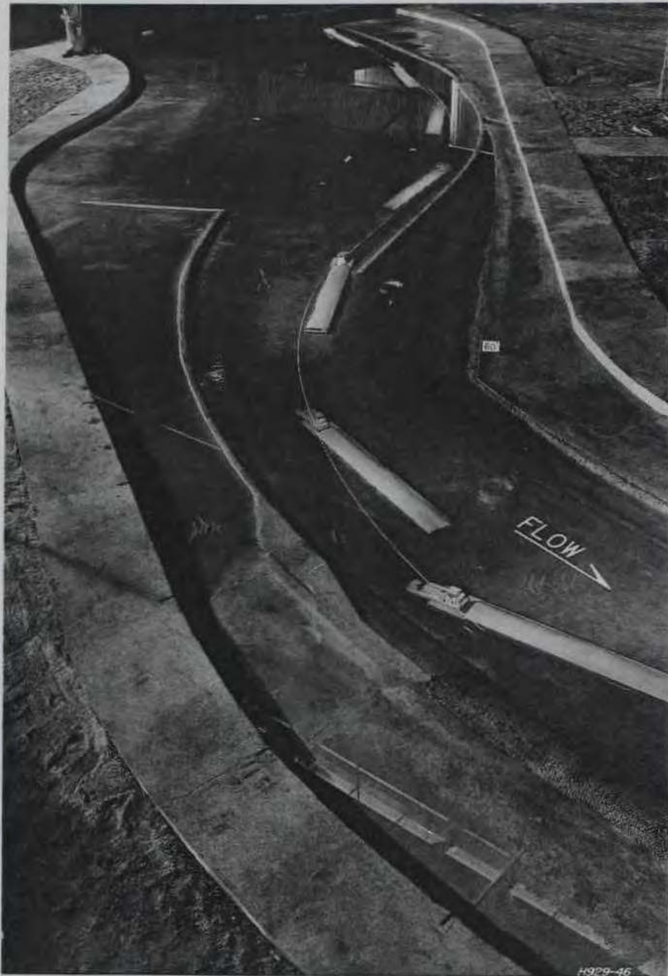
Photo 4. Plan B, looking upstream, discharge 60,000 cfs. Path of down-bound tow entering Piermont cutoff. Note tendency for tow to be confined against right descending bank
