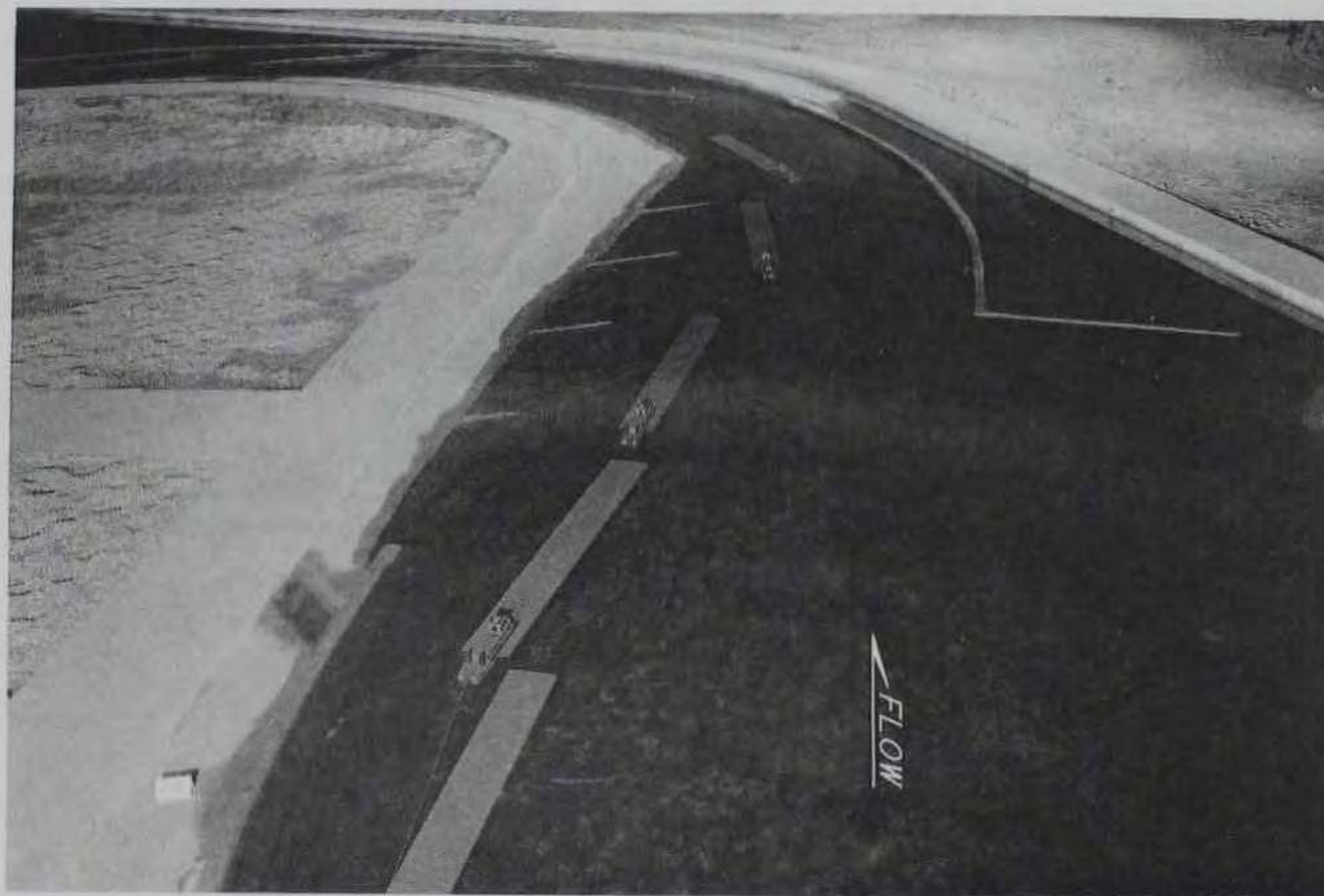
Photo 12. Plan C, looking downstream, discharge 60,000 cfs. Path of downbound tow driving past four spur dikes and into Piermont cutoff
