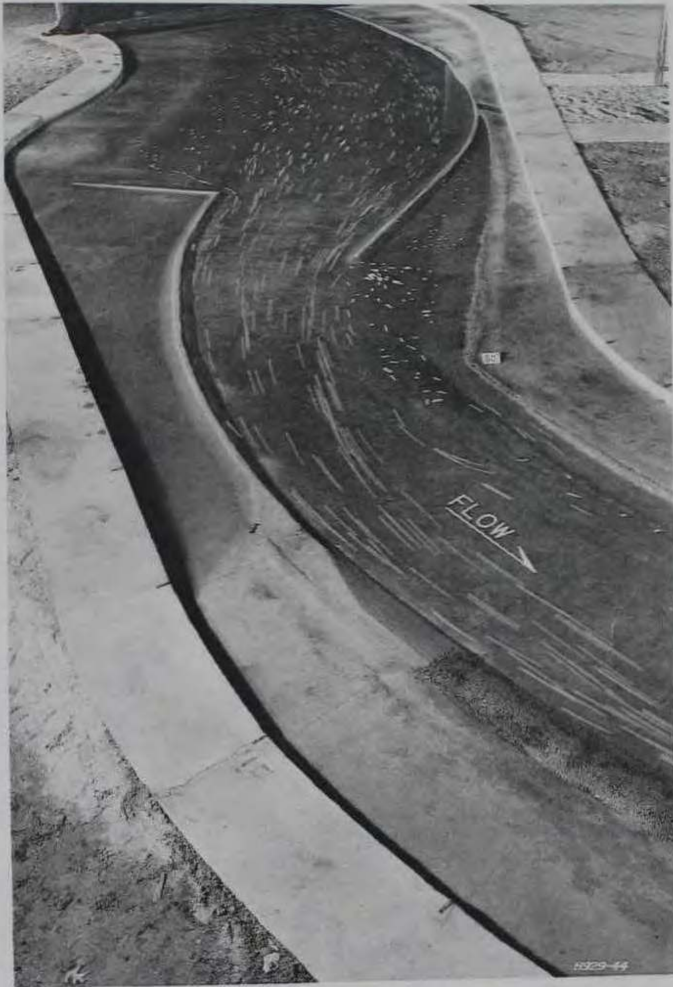
Photo 1. Plan B, looking upstream, discharge 60,000 cfs. Confetti showing surface current patterns entering and through Piermont cutoff
