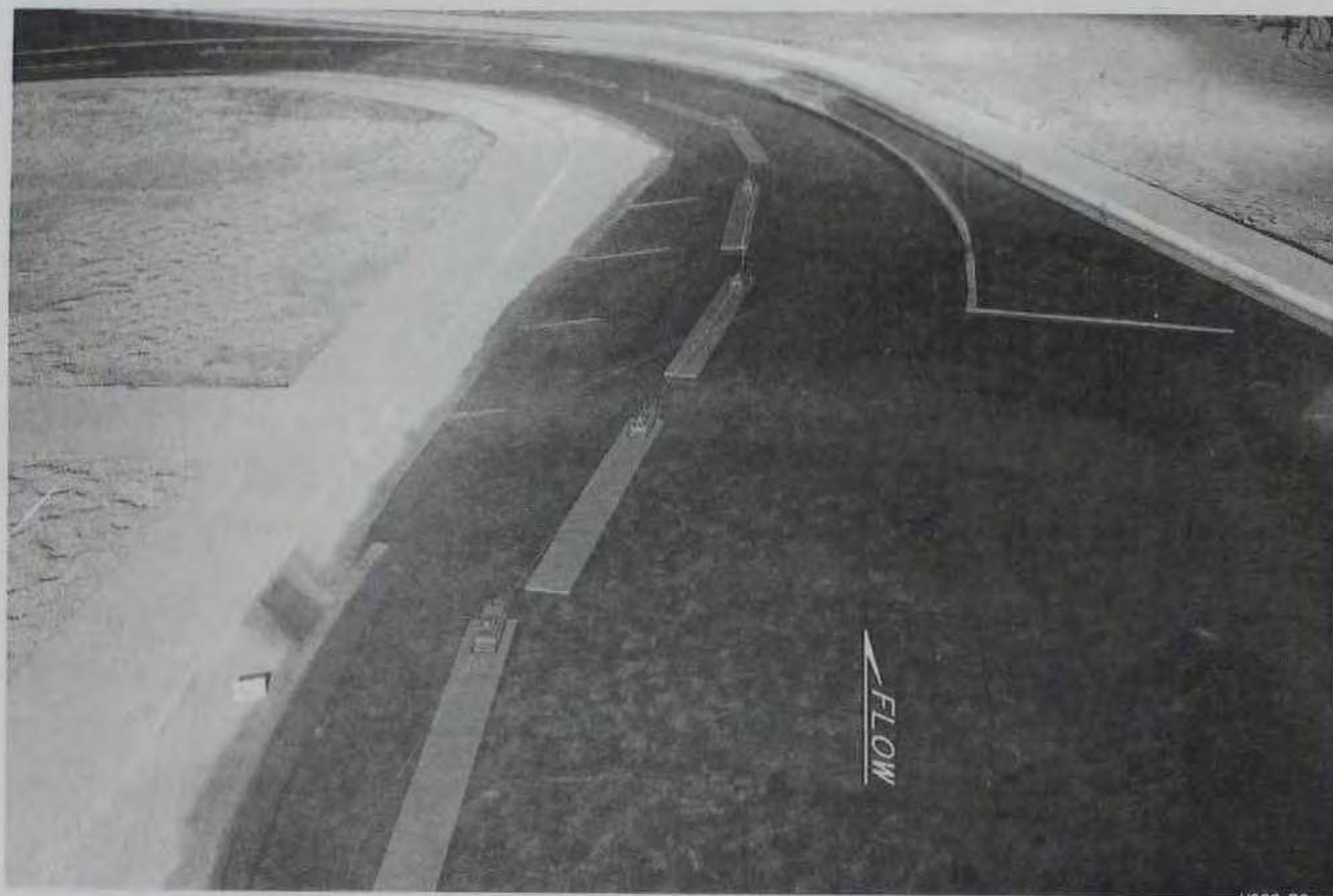
Photo 14. Plan C, looking downstream, discharge 80,000 cfs. Path of upbound tow leaving Piermont cutoff
