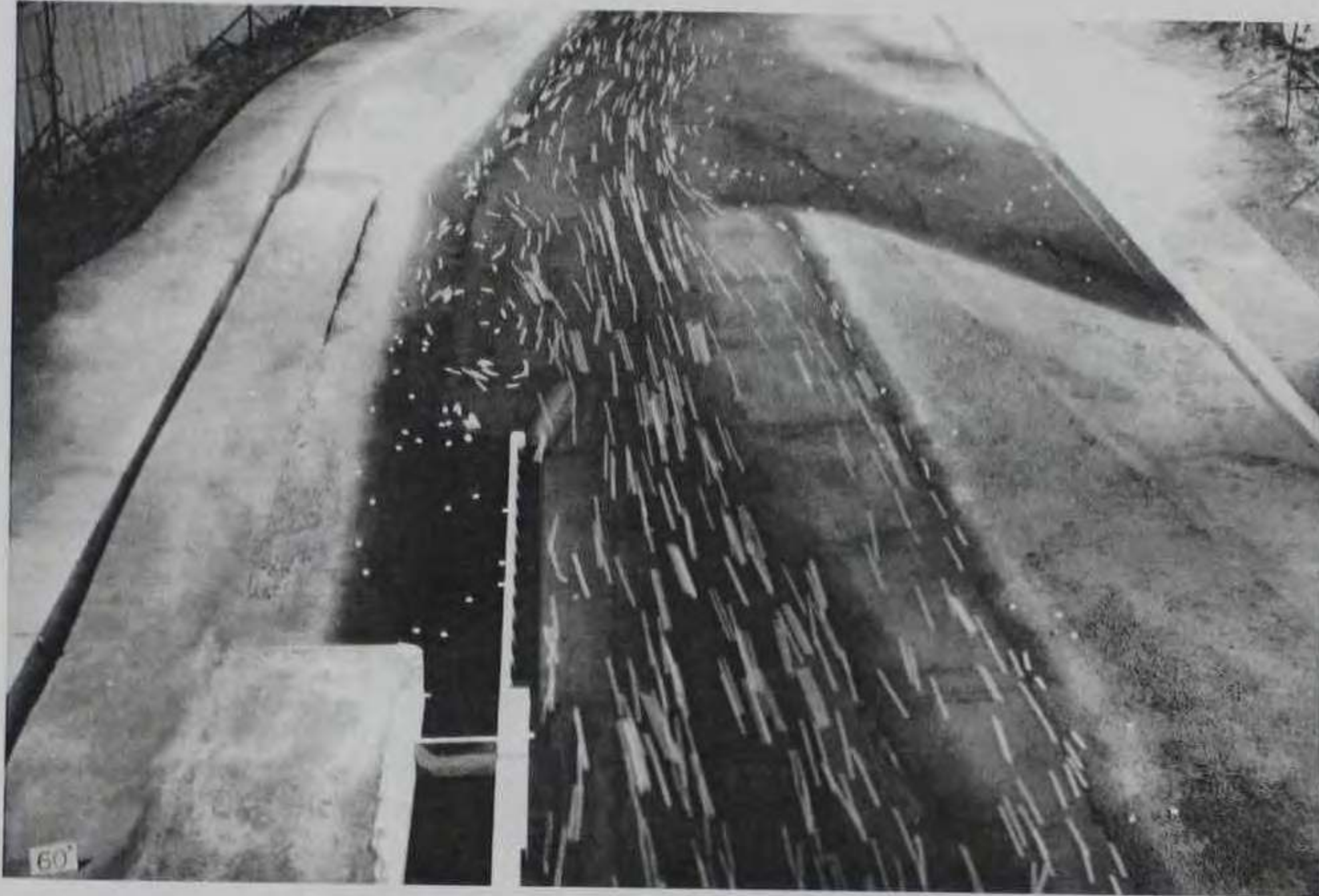
Photo 28. Plan D, looking downstream, discharge 60,000 cfs. Confetti showing surface current patterns
