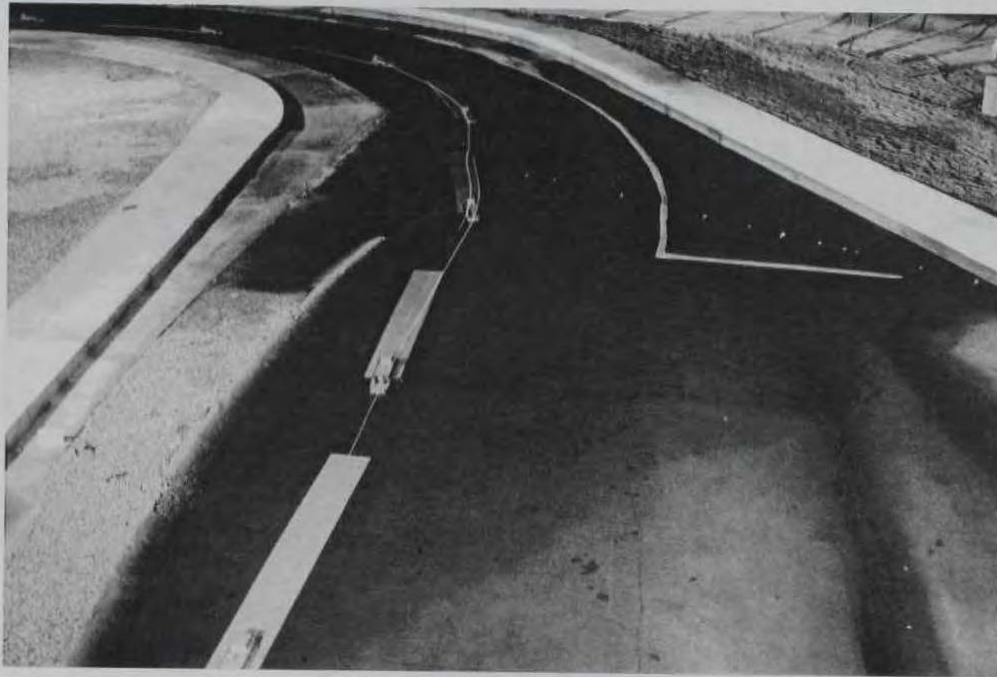
Photo 30. Plan D, looking downstream, discharge 80,000 cfs. Path of downbound tow flanking past Bull Revetment and into Piermont cutoff. Note tendency for currents to move toward left bank in vicinity of Piermont cutoff
