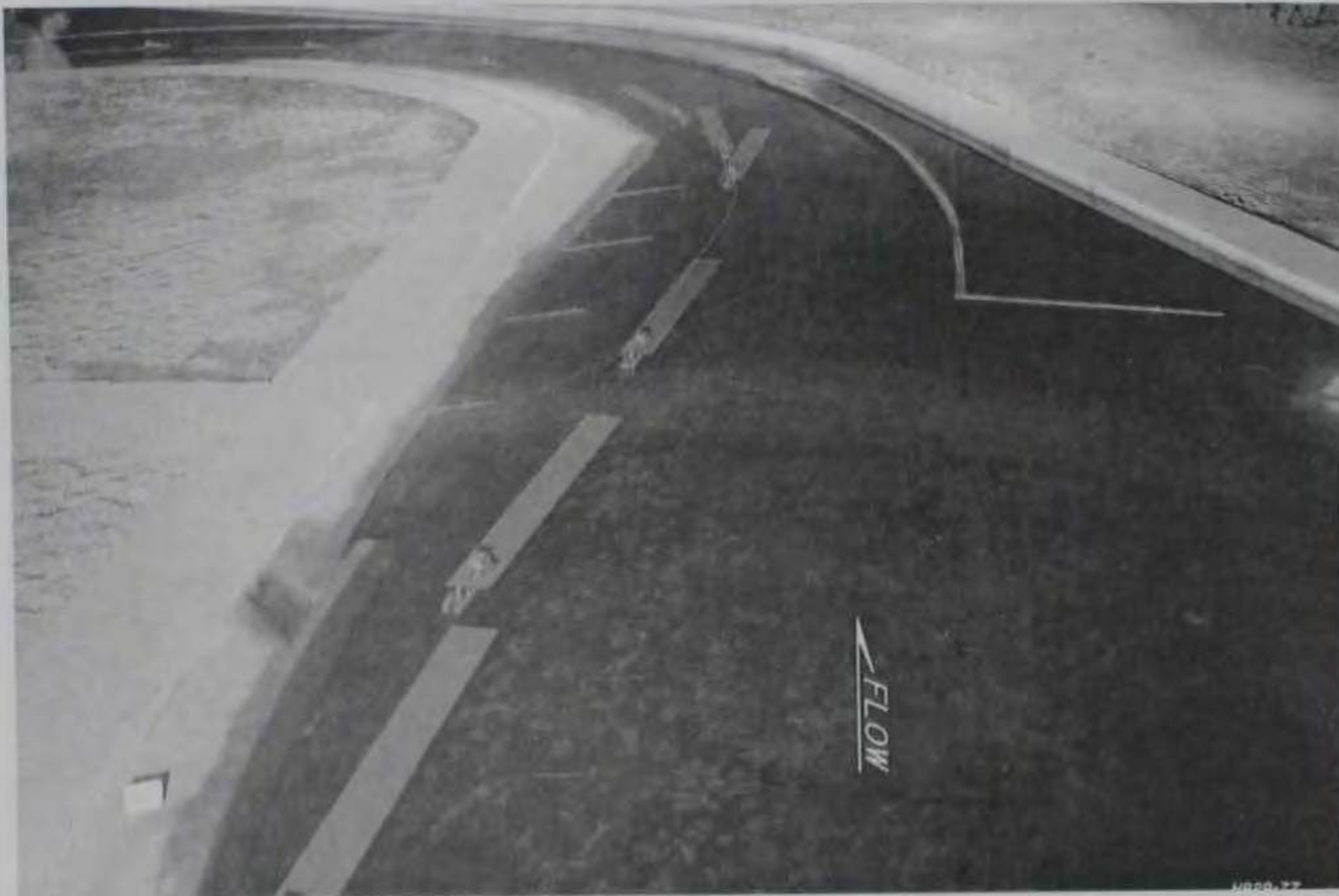
Photo 13. Plan C, looking downstream, discharge 80,000 cfs. Path of downbound tow flanking past four spur dikes and into Piermont cutoff. Note that tow is positioned to inside of bend
