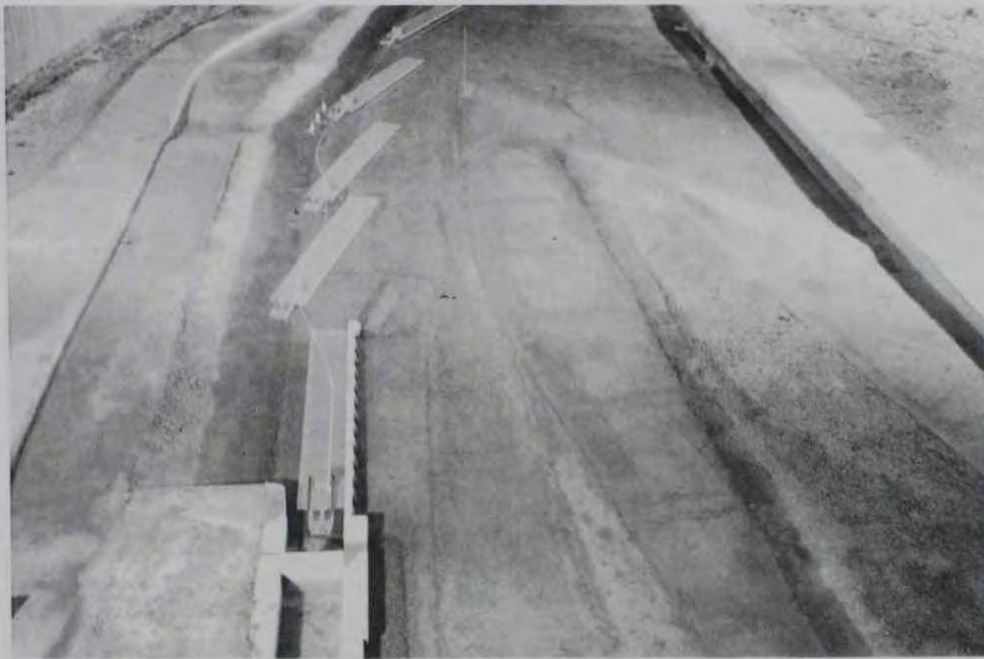
Photo 35. Plan D, looking downstream, discharge 80,000 cfs. Path of downbound tow leaving the lower lock approach. Note tendency for currents to move toward left bank and into mooring dolphins
