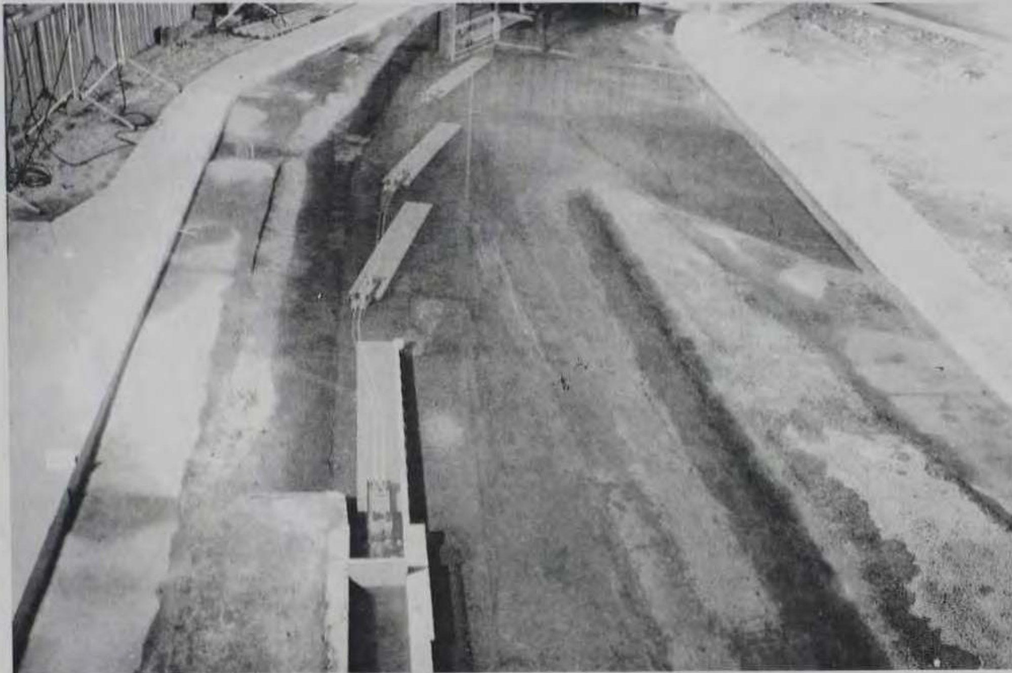
Photo 39. Plan D-2, looking downstream, discharge 80,000 cfs. Path of downbound tow leaving the lower lock approach
