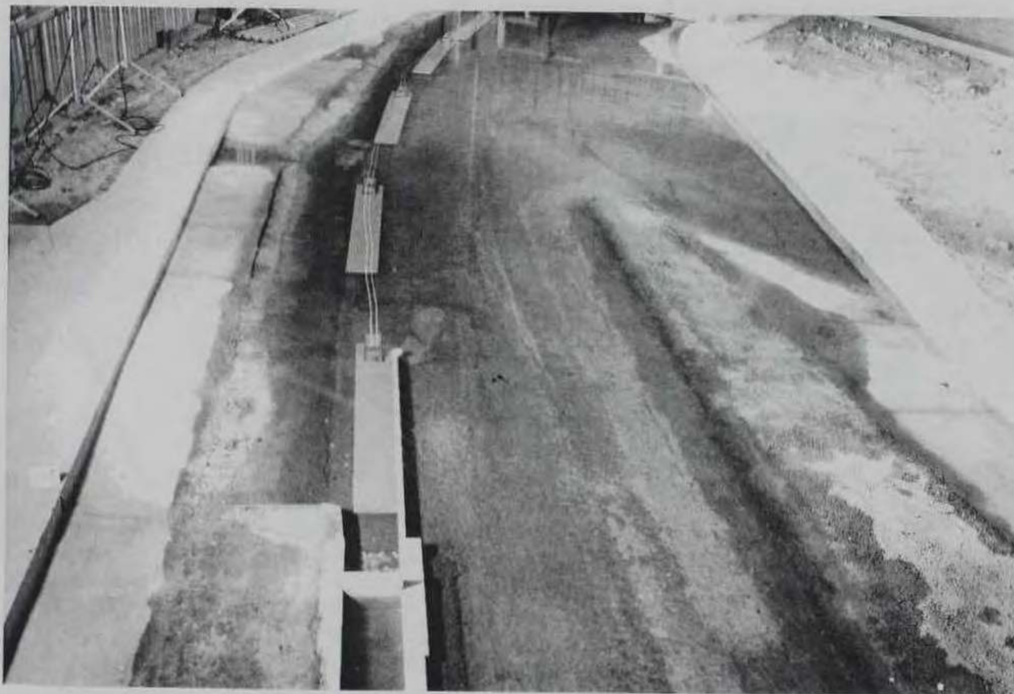
Photo 40. Plan D-2, looking downstream, discharge 134,000 cfs. Path of upbound tow entering the lower lock approach
