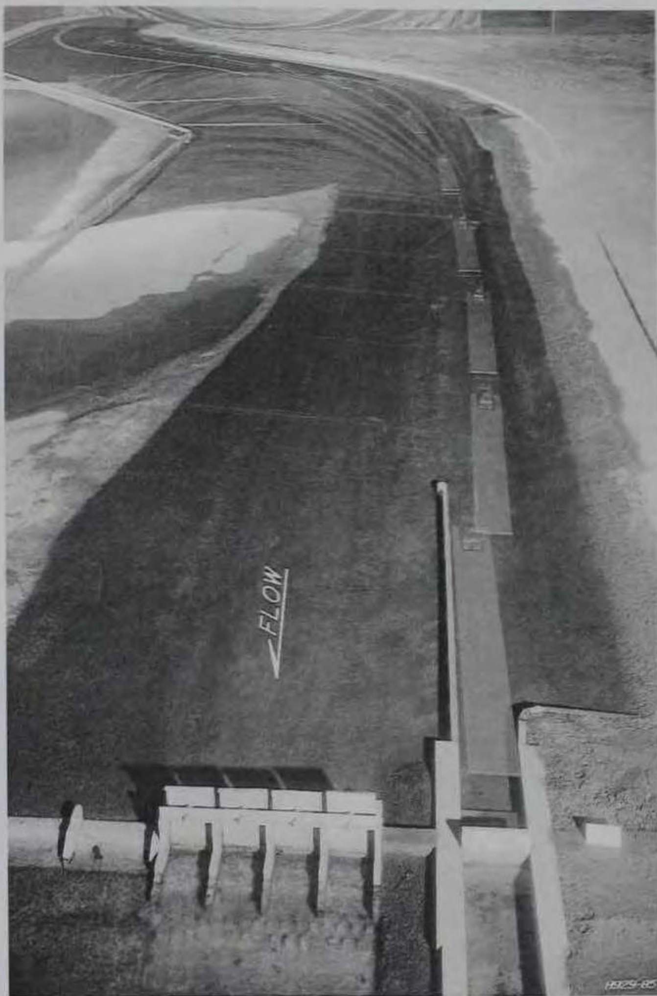
Photo 21. Plan C-2, looking upstream, discharge 60,000 cfs. Path of downbound tow entering the upper lock approach
