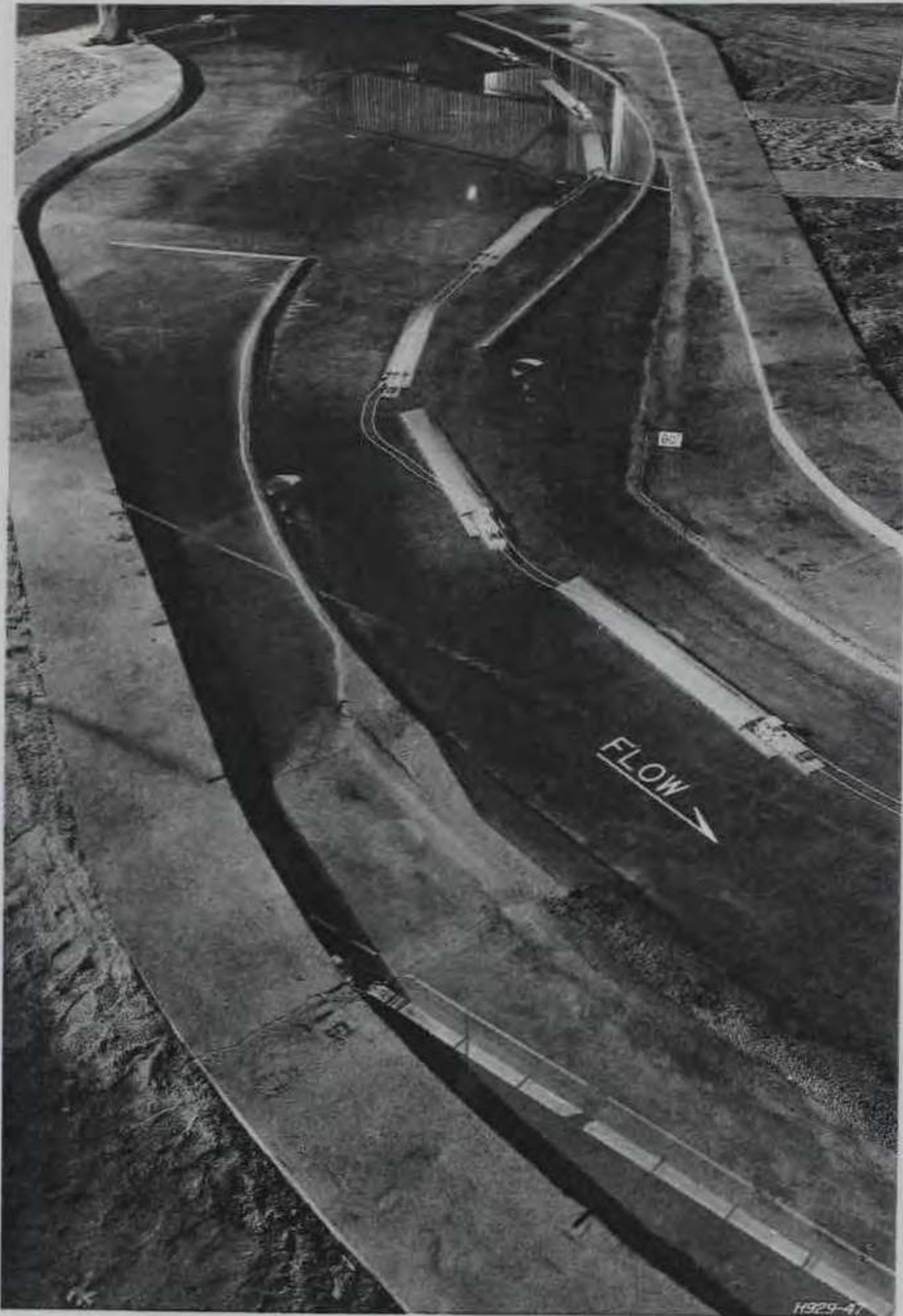
Photo 6. Plan B, looking upstream, discharge 60,000 cfs. Path of upbound tow leaving Piermont cutoff. Note maneuvering near end of Bull Revetment
