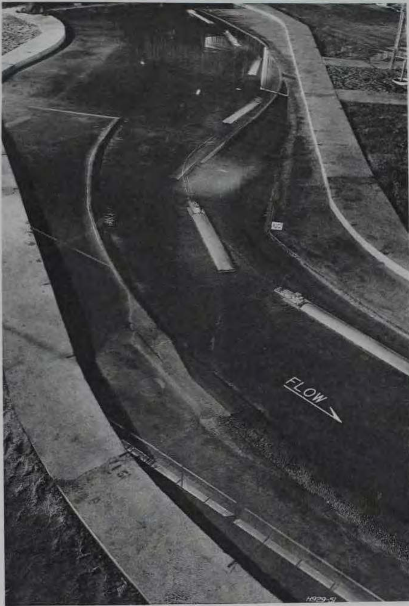
Photo 5. Plan B, looking upstream, discharge 100,000 cfs. Path of down-bound tow flanking into Piermont cutoff
