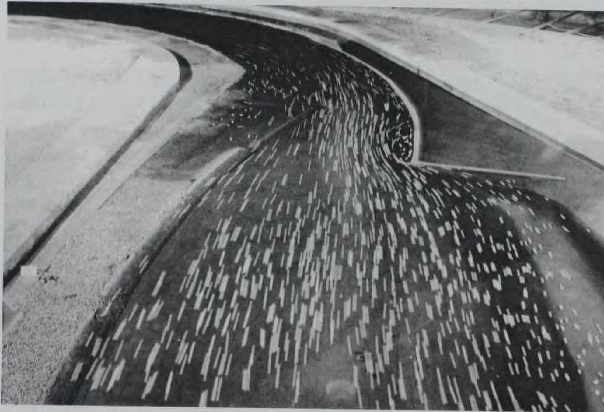
Photo 26. Plan D, looking downstream, discharge 80,000 cfs. Confetti showing surface current patterns
