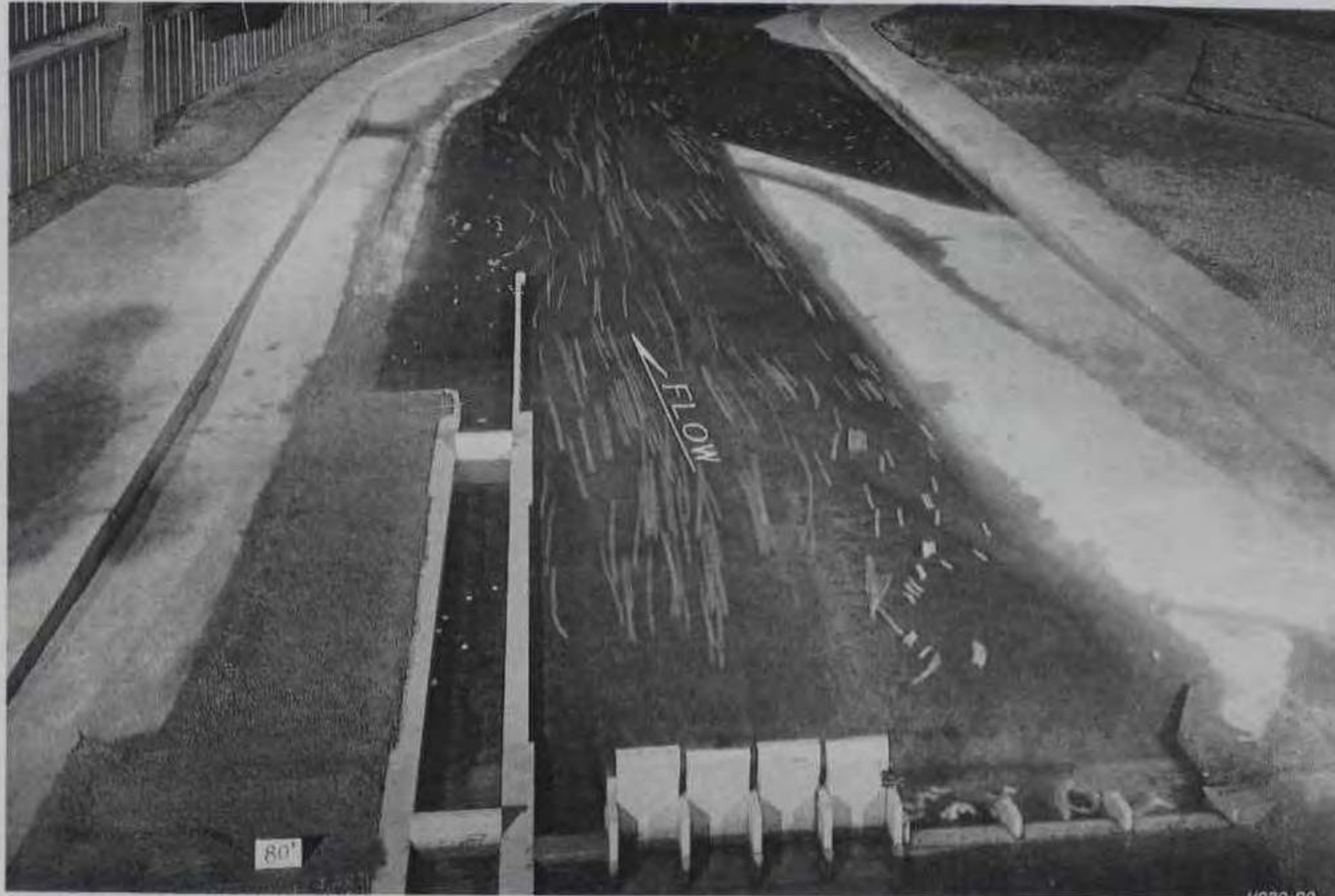
Photo 16. Plan C-1, looking downstream, discharge 80,000 cfs. Confetti showing surface current patterns in the lower lock approach. Note eddy downstream of guard wall
