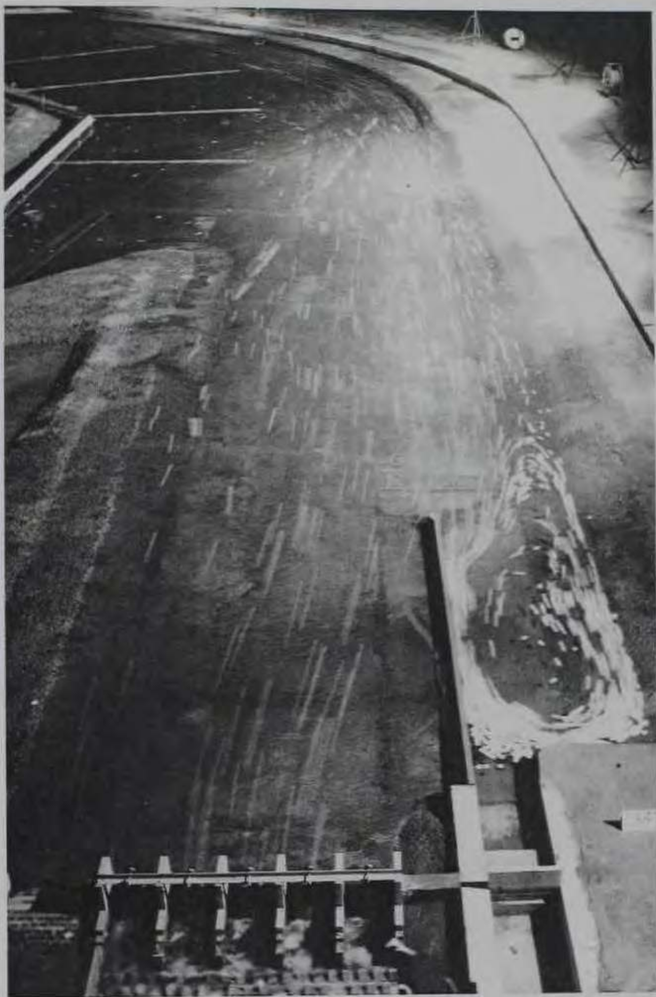
Photo 27. Plan D, looking upstream, discharge 134,000 cfs. Confetti showing surface current patterns. Note large eddy landward of guard wall
