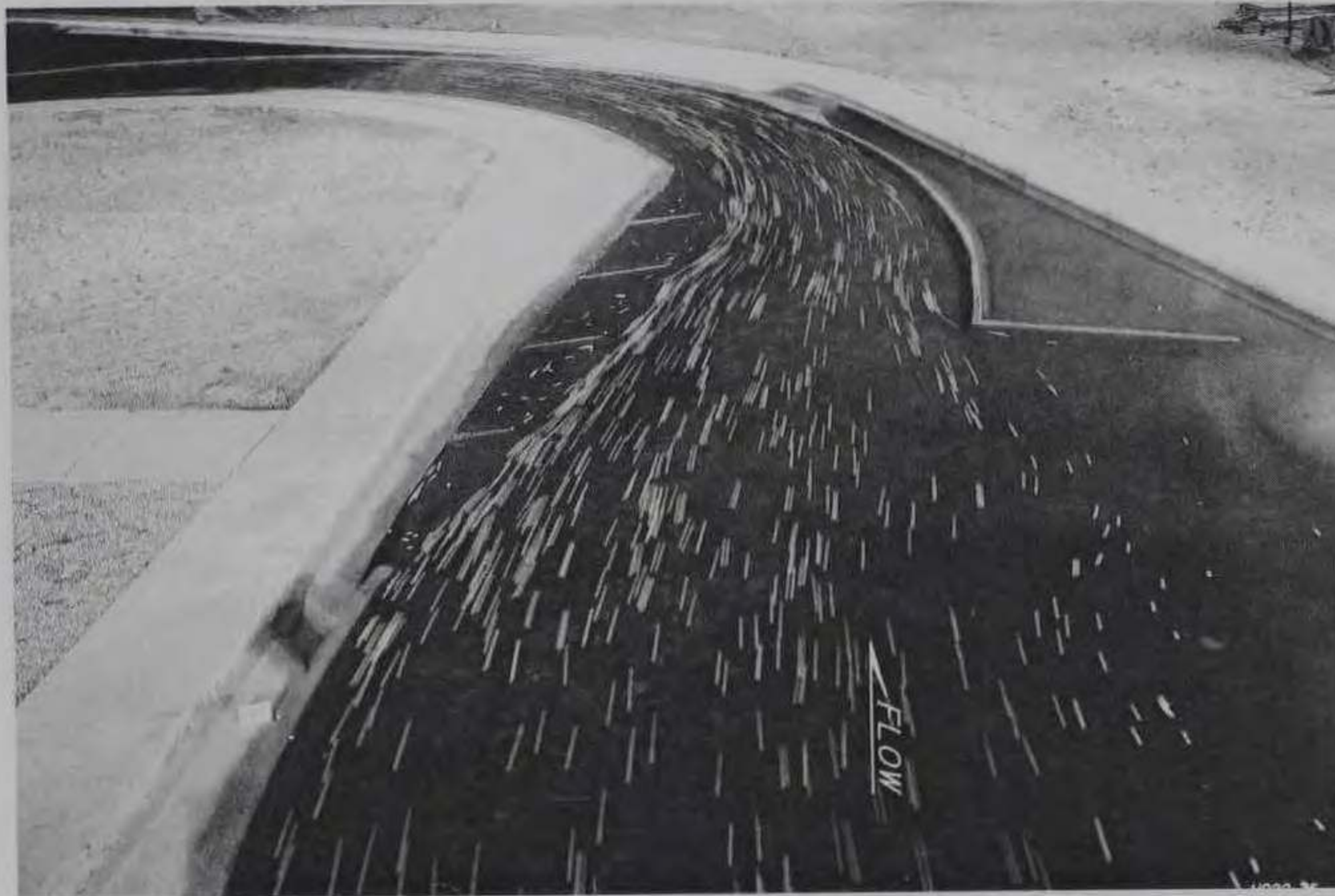
Photo 11. Plan C, looking downstream, discharge 80,000 cfs. Confetti showing surface current patterns entering and through Piermont cutoff
