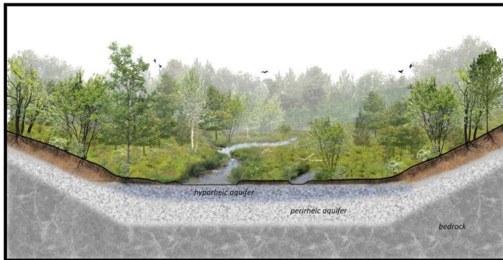
FIGURE 6 | Schematic representation of a fully connected stream corridor where biogeomorphic processes (e.g. large wood, beaver, vegetation) and river-wetland attributes (e.g. valley geometry, channel planforms, channel migration, hyporheic and regional aquifers) interact in complex ways, via multiple, nested feedback loops. Original illustration provided by LandStudies, Inc., Pennsylvania (with permission from Land Studies, 2021).
