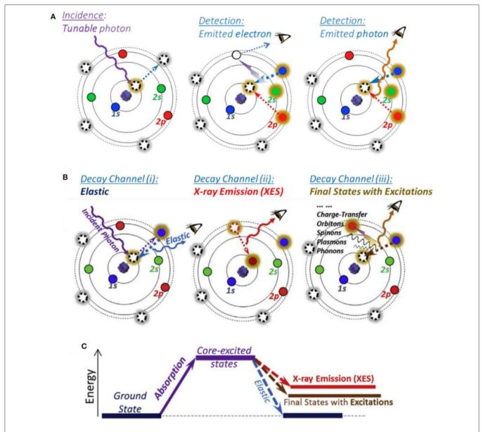
FIGURE 1 | Atomic schematic of soft X-ray spectroscopy (SXS). (A) sXAS excitation and decay processes with electron and photon detection modes. (B) Different decay channels leading to various features generated on mapping of resonant inelastic X-ray scattering (mRIXS). (C) Three types of final states. Reprinted from Yang et al. (2013) and Yang and Devereaux (2018), with permission respectively from Elsevier.
