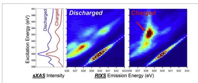
FIGURE 5 | Soft X-ray absorption spectroscopy (sXAS) and mapping of resonant inelastic X-ray scattering (mRIXS) data collected on charged and discharged anode material Na<sub>2.05</sub>Mn[Mn<sup>I</sup>(CN)<sub>6</sub>]<sub>0.81</sub> and Na<sub>1.24</sub>Mn[Mn<sup>II</sup>(CN)<sub>6</sub>]<sub>0.81</sub>. Reprinted from Yang and Devereaux (2018) with permission from Elsevier.
