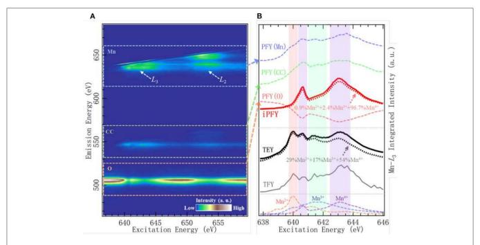
FIGURE 4 | Mn-L mapping of resonant inelastic X-ray scattering (mRIXS) (A) and various absorption profiles (B) of Na<sub>0.6</sub>Li<sub>0.2</sub>Mn<sub>0.8</sub>O<sub>2</sub>. Reproduced from Wu et al. (2020b) with no permission required from authors.
