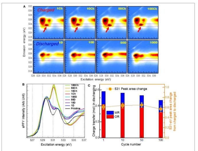
FIGURE 7 | Evaluation of reversibility and cyclability of O redox upon extended cycles. (A) O-K mapping of resonant inelastic X-ray scattering (mRIXS) and (B) super-partial fluorescence yield (sPFY) of charged and discharged electrodes after the 1st, 10th, 50th, and 100th cycles. (C) Quantification of the capacity contribution from O and Mn redox in the unit of charge transfer. Reprinted from Dai et al. (2019) with permission from Elsevier.
