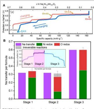
**FIGURE 9** | Electrochemistry and redox activities in  $Na_{2/3}Ni_{1/3}Mn_{2/3}O_2$  (NNMO). **(A)** Electrochemical profile of NNMO with negligible voltage hysteresis. **(B)** Quantitative evaluation on the electrochemical capacity from TM and O redox. Reprinted from Dai et al. (2020) with permission from *Nano Energy*.
