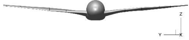
Fig. 15 Front view of the generic aircraft configuration. Wing is twisted at five section cuts depicted by the black lines. The left and the right wing show the maximum positive and negative twists, respectively.
