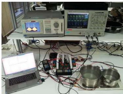
Fig. 12. Experimental induction heating prototype.
