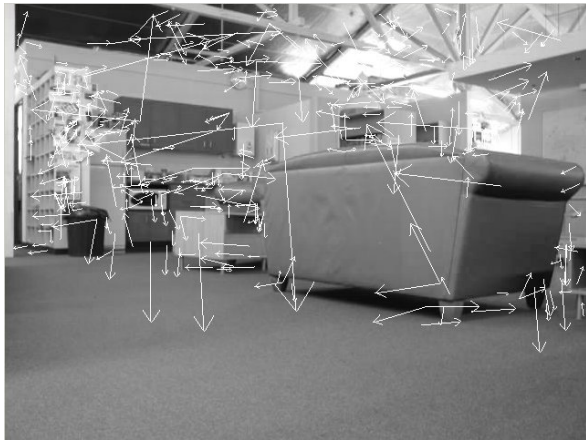
Figure 1: Typical indoor office environment and the extracted SIFT features with their locations represented by arrows. The length of the arrow represent the scale of the extracted keypoint and the direction represents the orientation of the descriptor.
