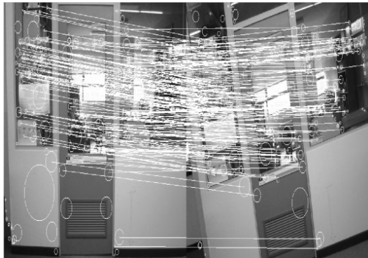
Figure 5: Keypoint matching between images rotated 17 degrees. Even under significant rotation 66 key points were matched, approximately 20 percent of the keypoints generated for the image.
