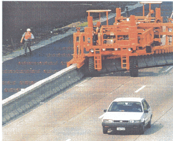
FIGURE 5 Machine to place movable barrier in setting up a lane closure (Rathbone 2000).
