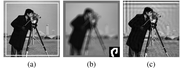
Fig. 1. Illustration of the boundary artifacts. (a) The latent clear image of size 256 \times 256 with FOV shown in the white box. (b) Synthetic blurred image using a PSF of size 20 \times 20 (shown at its bottom-right corner), where the missing boundary information is padded with the mean value of the whole image. (c) Restored image with severe boundary visual artifacts.
